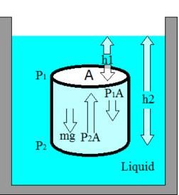
(A) and height  $(h_2-h_1)$ . P1, P2 pressures as the liquid is in static equilibrium and the net force acting on it is zero.
