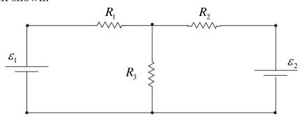
$\varepsilon_1$  = 8 volt,  $\varepsilon_2$  = 4 volt,  $R_1$  = 1 K $\Omega$ ,  $R_2$  = 2 K $\Omega$ ,  $R_3$  = 4 K $\Omega$ .
