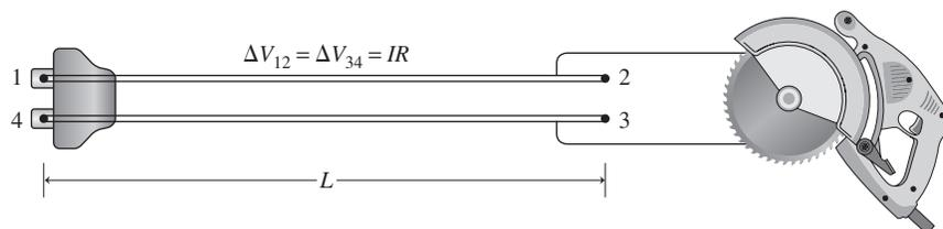
The copper wires in the extension cord will produce a voltage drop due to their resistance:  $\Delta V_{12} = \Delta V_{34} = IR$ . The resistance is given by Equation 24.6:  $R = \rho L / A$ , where  $\rho = 1.68 \times 10^{-8} \Omega \cdot \text{m}$  for copper,  $A$  is the area of the 1-mm-wide wire, and  $L$  is the length of the cord. For the voltage differences to be consistent with each other:
