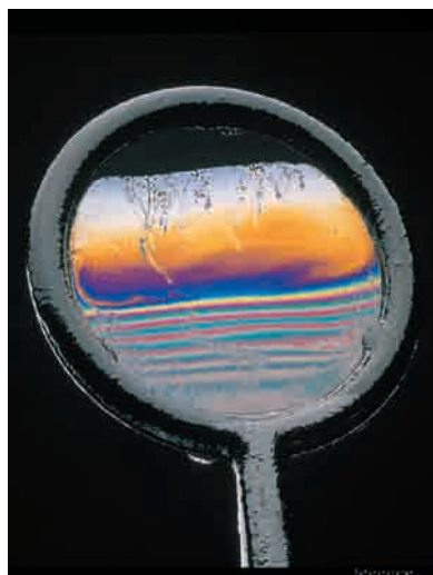
Fig. 35-18 The reflection of light from a soapy water film spanning a vertical loop. The top portion is so thin that the light reflected there undergoes destructive interference, making that portion dark. Colored interference fringes, or bands, decorate the rest of the film but are marred by circulation of liquid within the film as the liquid is gradually pulled downward by gravitation. (Richard Megna/Fundamental Photographs)
