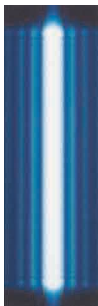
Fig. 36-1 This diffraction pattern appeared on a viewing screen when light that had passed through a narrow vertical slit reached the screen. Diffraction caused the light to flare out perpendicular to the long sides of the slit. That flaring produced an interference pattern consisting of a broad central maximum plus less intense and narrower secondary (or side) maxima, with minima between them. (Ken Kay/ Fundamental Photographs )
