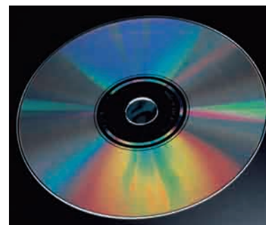
The fine rulings, each 0.5 \mu\text{m} wide, on a compact disc function as a diffraction grating. When a small source of white light illuminates a disc, the diffracted light forms colored “lanes” that are the composite of the diffraction patterns from the rulings. (Kristen Brochmann/Fundamental Photographs)
