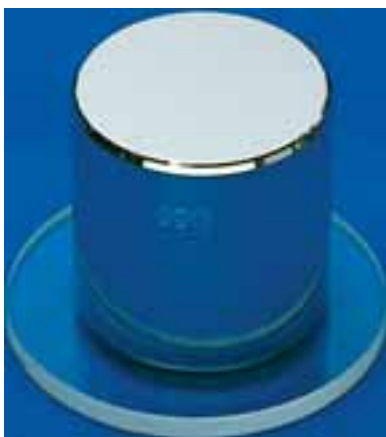
Fig. 1-3 The international 1 kg standard of mass, a platinum–iridium cylinder 3.9 cm in height and in diameter. (Courtesy Bureau International des Poids et Mesures, France)
