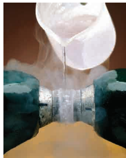
Liquid oxygen is suspended between the two pole faces of a magnet because the liquid is paramagnetic and is magnetically attracted to the magnet. (Richard Megna/Fundamental Photographs)
