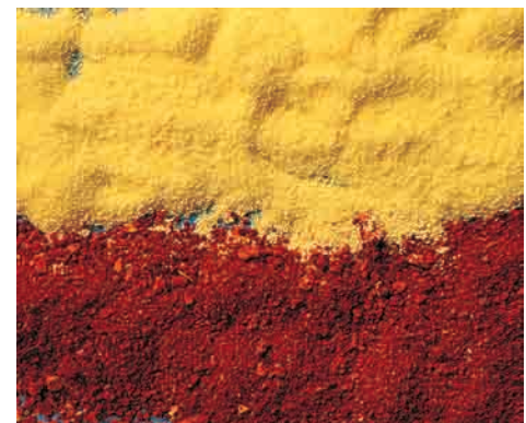
Fig. 39-10 Two samples of powdered cadmium selenide, a semiconductor, differing only in the size of their granules. Each granule serves as an electron trap. The lower sample has the larger granules and consequently the smaller spacing between energy levels and the lower photon energy threshold for the absorption of light. Light not absorbed is scattered, causing the sample to scatter light of greater wavelength and appear red. The upper sample, because of its smaller granules, and consequently its larger level spacing and its larger energy threshold for absorption, appears yellow. (From Scientific American , January 1993, page 122. Reproduced with permission of Michael Steigerwald, Bell Labs–Lucent Technologies)
