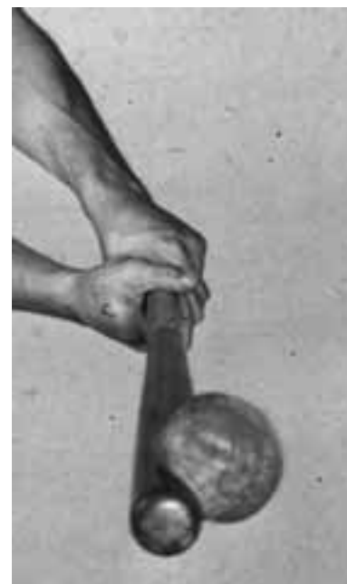
The collision of a ball with a bat collapses part of the ball. (Photo by Harold E. Edgerton. ©The Harold and Esther Edgerton Family Trust, courtesy of Palm Press, Inc.)
