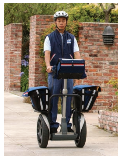
Fig. 11-1 The self-righting Segway Human Transporter. (Justin Sullivan/Getty Images News and Sport Services)
