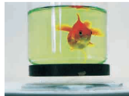
A disk-shaped magnet is levitated above a superconducting material that has been cooled by liquid nitrogen. The goldfish is along for the ride. (Courtesy Shoji Tonaka/International Superconductivity Technology Center, Tokyo, Japan)
