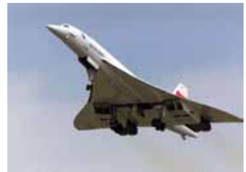
Fig. 18-9 When a Concorde flew faster than the speed of sound, thermal expansion due to the rubbing by passing air increased the aircraft’s length by about 12.5 cm. (The temperature increased to about 128^{\circ}\text{C} at the aircraft nose and about 90^{\circ}\text{C} at the tail, and cabin windows were noticeably warm to the touch.) (Hugh Thomas/BWP Media/Getty Images News and Sport Services)
