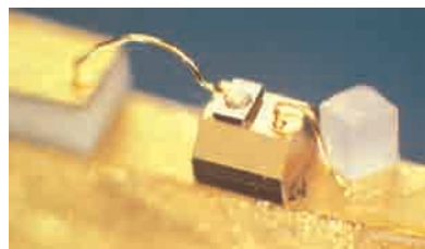
Fig. 41-18 A junction laser developed at the AT&T Bell Laboratories. The cube at the right is a grain of salt. (Courtesy AT&T Archives and History Center, Warren, NJ)
