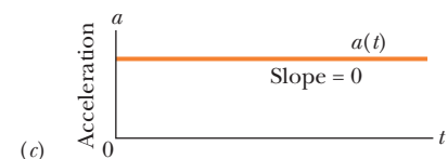
Figure 2-9 (a) The position x(t) of a particle moving with constant acceleration. (b) Its velocity v(t) , given at each point by the slope of the curve of x(t) . (c) Its (constant) acceleration, equal to the (constant) slope of the curve of v(t) .
