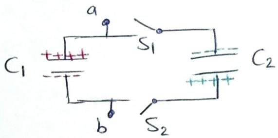
After the switches are closed, the potential differences across the capacitors are the same and they are connected in parallel.
