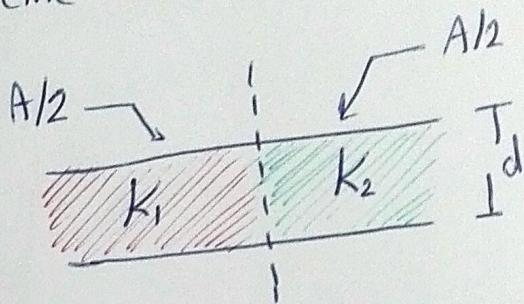
$\Rightarrow$  Consider the two capacitors are in parallel  $\Rightarrow C_{eq} = C_1 + C_2$
