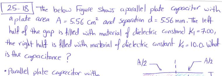
· Parallel plate capacitor with dielectric material C= KEA
