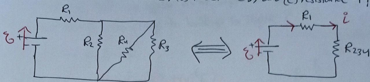
$R_2$ ,  $R_3$  and  $R_4$  are all in parallel
