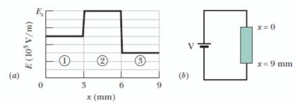
• Same material => Same resistivity for the three sections  $\vec{E} = P\vec{J} \Rightarrow P = \vec{E} \Rightarrow \vec{E}_1 = \vec{E}_2 = \vec{E}_3 \qquad (\note)$ From the Figure (a) =>  $\vec{E}_1 = 5 \times 10^3 \text{ V/m}$   $\vec{E}_2 = 8 \times 10^3 \text{ V/m}$  $\vec{E}_3 = 3 \times 10^3 \text{ V/m}$
