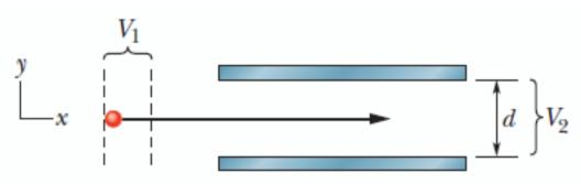
a) Electron travels in astraight line in the gap
