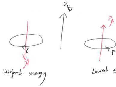
$$\Rightarrow V = \begin{cases} 0, & \Theta = 90 \\ MB, & \Theta = 180^{\circ} \text{ anti-parallel} \\ -MB, & \Theta = 0^{\circ} \text{ parallel} \end{cases}$$
