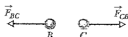
(b) The force on B due to C has the same magnitude as the force on C due to B .
