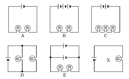
42. In the diagrams, all light bulbs are identical and all emf devices are identical. In which circuit (A, B, C, D, E) will the bulbs be dimmest?
