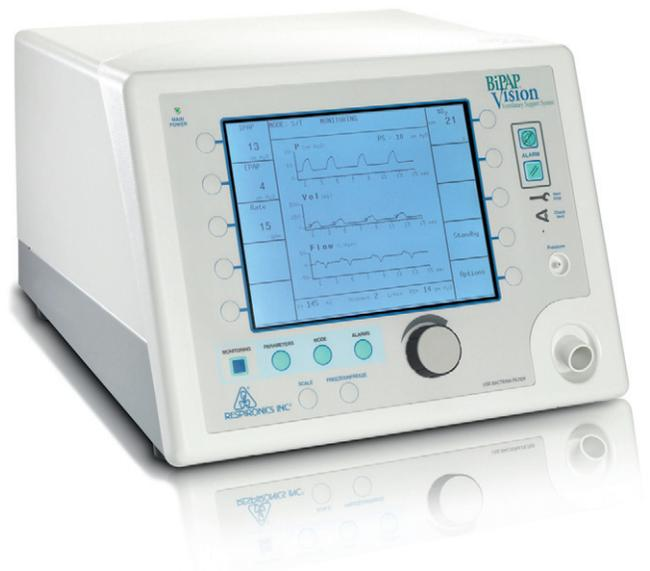
**FIGURE 9-33** Noninvasive positive-pressure ventilation (NPPV) may be administered through a mask with the BiPAP Vision ventilator. This ventilator is capable of operating in four modes: pressure support (PS); spontaneous/timed (S/T) mode, which is pressure support with backup pressure control; timed (T), which is pressure control; and continuous positive airway pressure (CPAP). (Courtesy Phillips Healthcare, Andover, Massachusetts.)
