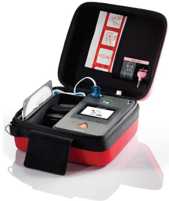
**FIGURE 10-9** Automated external defibrillator. (Courtesy Philips Healthcare, Bothell, Washington.)
