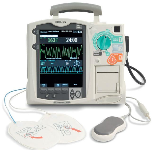
FIGURE 10-6 Defibrillator. (Courtesy Philips Healthcare, Andover, Massachusetts.)
