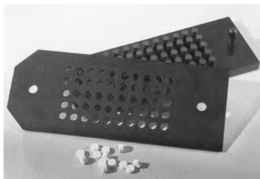
FIGURE 8.29 Laboratory mold for preparation of tablet triturates.
