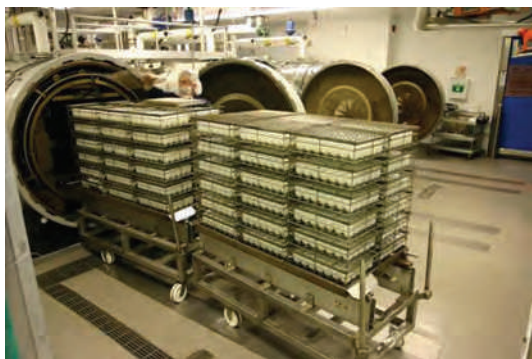
FIGURE 15.3 Autoclaving of IV electrolyte solutions. (Courtesy of Hospira, Inc.)
