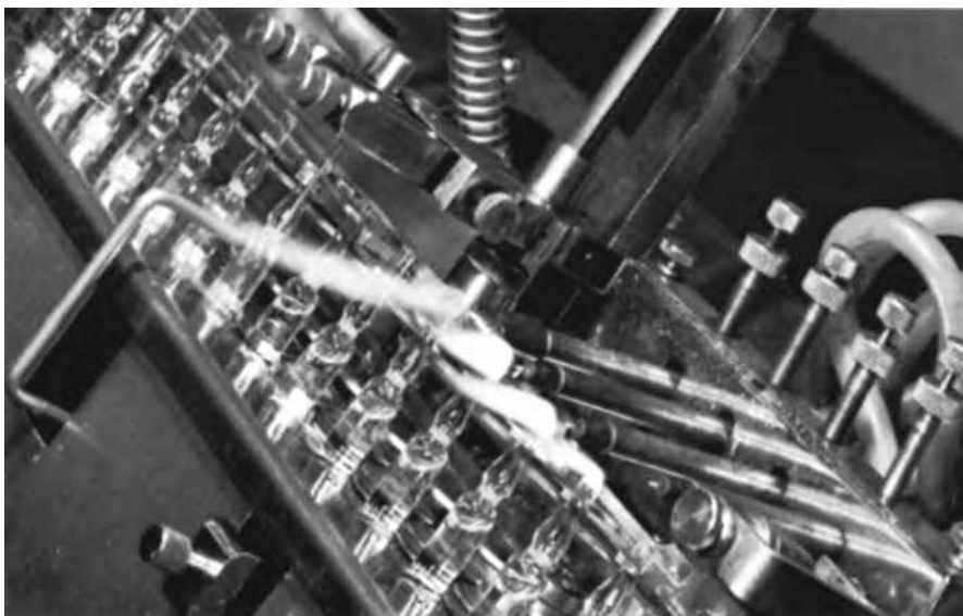
FIGURE 15.17 Ampul sealing. (Courtesy of Abbott Laboratories.)
