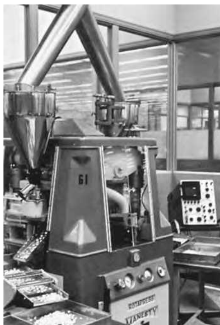
FIGURE 8.25 Manesty Rotapress rotary compression machine. Tablets leaving the machine run over a tablet duster to screen, where they are inspected. Material to be compressed is fed from the overhead hopper through yoke to the two compressing machine hoppers. Hardness of tablet is monitored electronically by oscilloscope at right. (Courtesy of Upjohn Company.)
