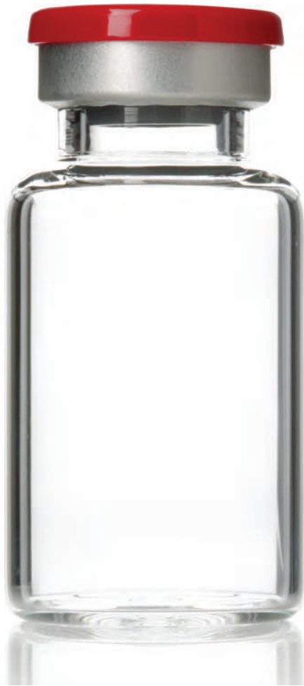
FIGURE 15.14 A typical vial for sterile injectable products, made from type I (borosilicate) glass. The rubber closure has been specially selected for compatibility with the product, desirable physical characteristics, and so on. The overseal holds the closure in place and provides ready access to the contents of the vial. (Courtesy of Hospira, Inc.)
