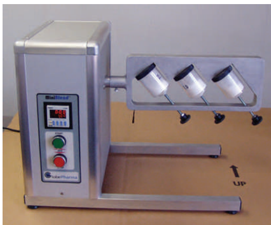
FIGURE 6.5 Laboratory-scale Triple V-type blender. (Courtesy of GlobePharma.)
