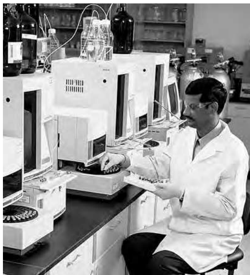
FIGURE 5.19 Assay of product samples using high-performance liquid chromatography. (Courtesy of Paddock Laboratories.)
