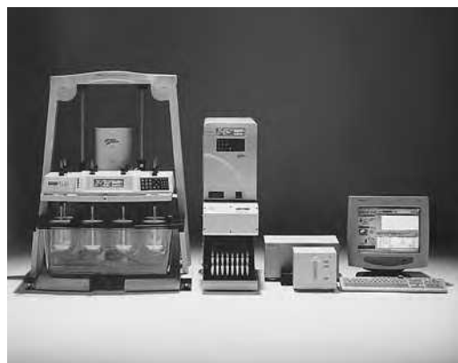
FIGURE 8.16 Hanson Automated Dissolution Test System. It features microprocessor and templates to create, edit, store, and validate dissolution protocols; graphical displays with menus; and icon-based program controls. (Courtesy of Hanson Research.)
