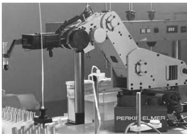
FIGURE 3.2 Robotics in laboratory use. Perkin-Elmer Robotic Arm and Perkin-Elmer Lambda 1a UV/VIS Spectrophotometer. (Courtesy of Elan Corporation, plc.)
