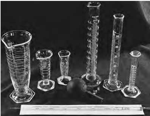
FIGURE C.5 Typical equipment for the pharmaceutical measurement of volume. Left: Conical graduates. Right: Cylindrical graduates. Front: A pipet for measurement of small volumes. Behind the pipet is a pipet filler used instead of the mouth to draw acids and other dangerous liquids into the pipet.
