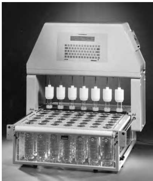
FIGURE 9.6 Varian Biodis Dissolution Apparatus for determining dissolution characteristics of modified-release products. (Courtesy of Varian Inc.)
