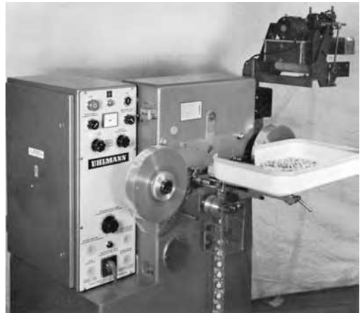
FIGURE 7.21 Strip packager for unit-dose dispensing of solid dosage forms. Drug information is imprinted on each package unit. This model has a fully automatic cutoff for 1 to 24 dosage units and is especially suited to unit-dose packaging and dispensing in hospitals, dispensaries, nursing homes, and clinics. (Courtesy of Lakso Company.)
