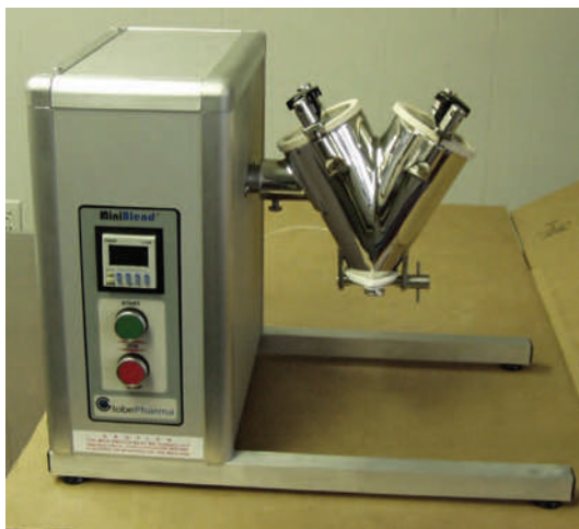
FIGURE 6.4 Laboratory-scale V-blender. (Courtesy of GlobePharma.)
