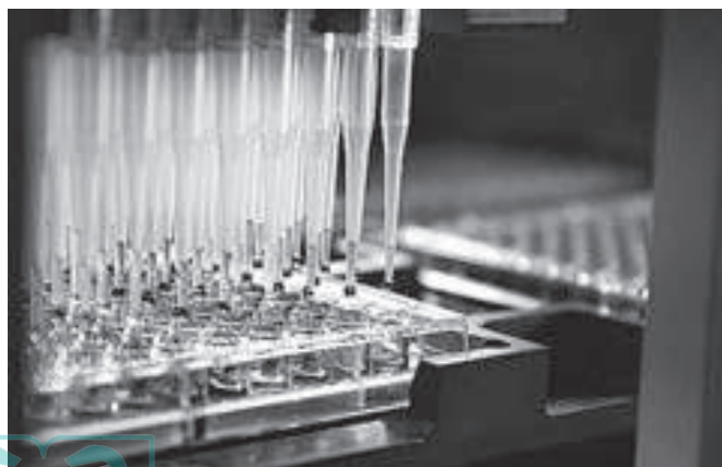
FIGURE 7.1 A pipetting robot system for fully automated high-throughput screening arrays.
