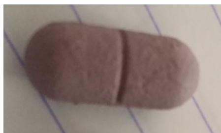
Figure 2: Orange peel effect and erosion
