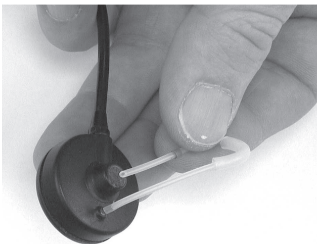
Figure 4.18 Positioning of the probe microphone against the control microphone during calibration.
