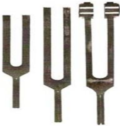
FIGURE 2.3 Several tuning forks. The larger forks vibrate at lower frequencies (produce lower-pitched tones) than the smaller forks.
