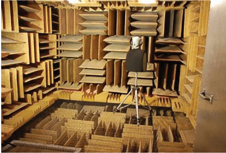
FIGURE 3.17 The inside of an anechoic chamber designed to eliminate sound reverberation. (Source: Orfield Laboratories.)
