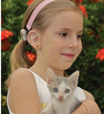
FIGURE 14.9 The vibrating receiver of a soft-band bone-conduction hearing aid sends sound waves to the cochlea through the bone-conduction auditory pathways of the skull. (Source: Oticon Medical.)
