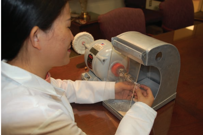
FIGURE 14.16 Earmolds and hearing aids can be ground and buffed when needed for greater physical comfort. The sound opening of the mold or hearing aid can be “belled” or scooped out to enhance high-frequency amplification, and vent openings can be enlarged to decrease the amount of low-frequency amplification.
