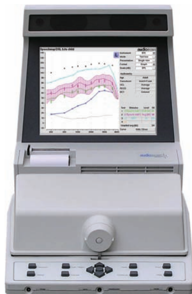
FIGURE 14.3 Hearing aid test system including sound chamber for 2 cm 3 electroacoustic analysis of hearing instruments and probe-microphone measurements. (Source: Audioscan.)
