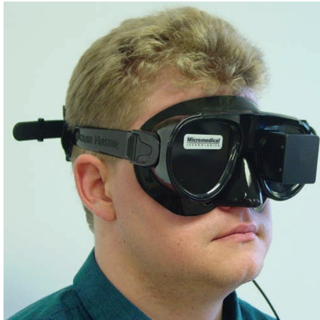
FIGURE 11.2 Specialized goggles allow for the observation and video recording of eye movement while testing the dizzy patient or while performing vestibular rehabilitation. (Source: Micromedical Technologies, 10 Kemp Drive, Chatham, IL 62629.)
