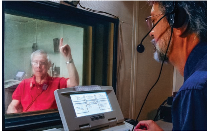
FIGURE 4.3 A commercial double-room sound-treated audiometric test chamber in use.
