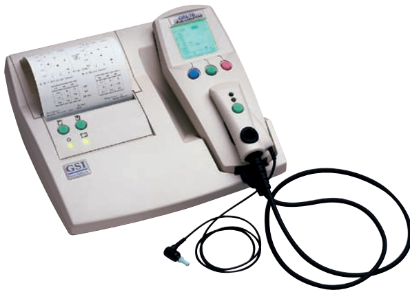
FIGURE 7.8 Commercial device for measurement of otoacoustic emissions, sounds generated by the cochlea indicative of cochlear function. (Source: Grason-Stadler Co.)
