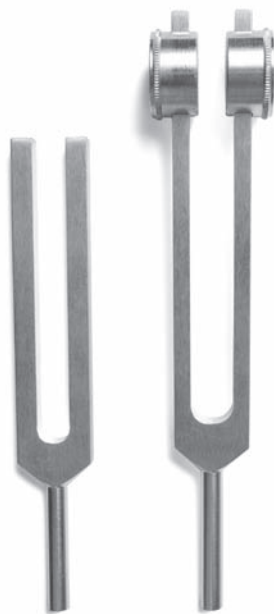
FIGURE 2.3 Several tuning forks. The larger forks vibrate at lower frequencies (produce lower-pitched tones) than the smaller forks. (Source: Fosterdesigns/iStock/360/Getty Images.)
