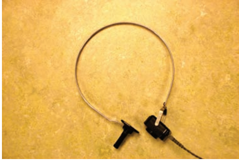
FIGURE 3.22 A bone-conduction vibrator through which pure tones may be routed using a pure-tone audiometer to measure bone-conduction sensitivity. (Source: Clark Audiology.)
