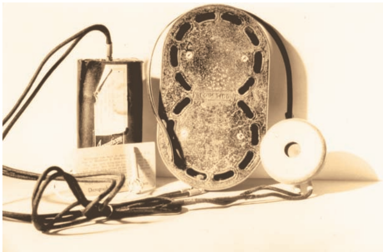
FIGURE 14.2 A complete carbon hearing aid consisting of a double carbon microphone for increased power, an earphone-style receiver with headband, and battery, circa 1910.
