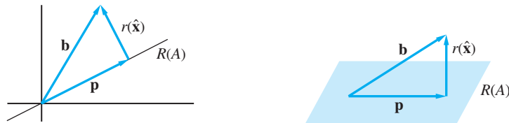
(a) \mathbf{b} \in R^2 and A is a 2 \times 1 matrix of rank 1. (b) \mathbf{b} \in R^2 and A is a 3 \times 2 matrix of rank 2.
