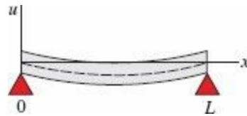
FIGURE 13.4.9 Simply supported beam in Problem 23
