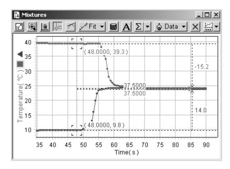
Since these two temp probes were not calibrated together first, I need to account for the offset.
