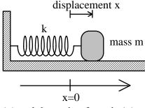
k is called the spring constant and is a measure of the stiffness of the spring. The minus sign indicates that the direction of the force is opposite to the direction of the displacement. In the SI system, the units of spring constant k are N/m. The diagram shows a mass to the right of its equilibrium position (x=0). The displacement of the mass is (+) and the spring force is to the left (-). If the spring is compressed, then x is
