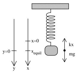
If the mass is hung from a vertical spring, it will still execute simple harmonic motion with the same period (5), as we will now show. When the mass is hung from the spring, the spring is stretched from its equilibrium length by the weight mg of the mass. The equilibrium displacement of the mass under the influence of the force of gravity (down) and the
