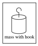
Remove the weight tray from the spring and load the spring with a 100 gram mass with a hook. Carefully, set the mass oscillating with a small amplitude motion and use a stop watch to time the interval for several complete oscillations. If the time for N complete periods (N  $\approx$  50 or more) is T<sub>total</sub>, then the period is T<sub>meas</sub> =  $\frac{T_{total}}{N}$ . By measuring the time for many periods, the uncertainty in T, due to your reaction time, is reduced by a factor of N.
