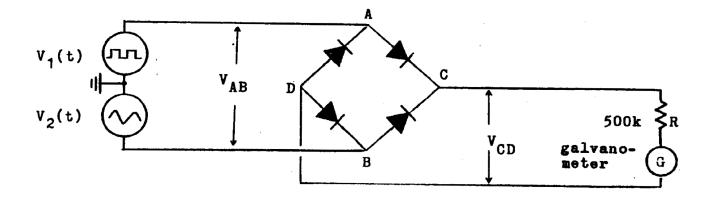
Prepare the apparatus: The previous circuit, two signal generators.
