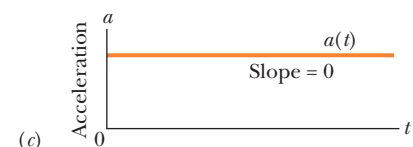
Figure 2-9 (a) The position x(t) of a particle moving with constant acceleration. (b) Its velocity v(t) , given at each point by the slope of the curve of x(t) . (c) Its (constant) acceleration, equal to the (constant) slope of the curve of v(t) .
