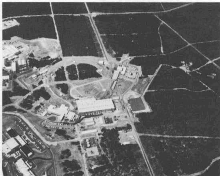
FIG. 8-25. Aerial view of the 33-GeV alternate gradient synchrotron at Brookhaven National Laboratory. The accelerating tunnel underground has a diameter of 840 ft. The building at "3 o'clock," the service, target, and experimental buildings, and at "9 o'clock" a 10-ton spark chamber. (Courtesy Brookhaven National Laboratory.)
