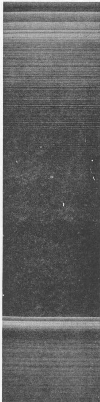
FIG. 12-9. A portion of the band spectrum of cyanogen (CN) in the ultraviolet. (Courtesy RCA Laboratories, Princeton, New Jersey.)
