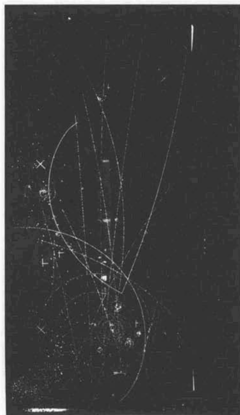
FIG. 11-9. A bubble-chamber photograph of a 3.3-GeV antiproton entering the bubble chamber from the bottom and colliding with a proton at point 1 to create a hyperon ( \Lambda^0 ) and an antihyperon ( \bar{\Lambda}^0 ). The \Lambda^0 particle decays into a proton and \pi^- pion at point 3; the \bar{\Lambda}^0 antiparticle into an antiproton and \pi^+ pion at point 2. (Courtesy Brookhaven National Laboratory.)
