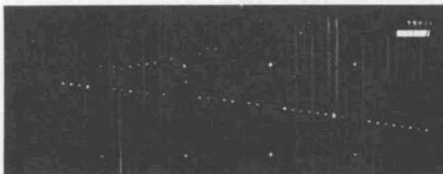
FIG. 8-10. Two tracks in a spark-chamber photograph used in experiments to establish the existence of the neutrino associated with the muon. (Courtesy Brookhaven National Laboratory.)
