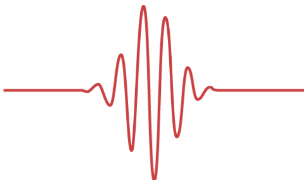
Figure 6.25 In this graphic, a particle is shown as a wave packet and its position does not have an exact value.
