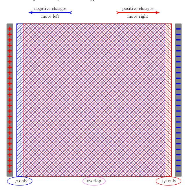
As the result of this move, the bulk of the dielectric — where the positive and negative charges continue to overlap each other — remains electrically neutral. But in a thin surface layer on the left side of the dielectric there are only negative charges, while in a similar layer on the right side there are only positive charges. Altogether, the dielectric's surfaces acquire non-zero net densities  $\sigma_b$  of bound charges as shown on the picture below:
