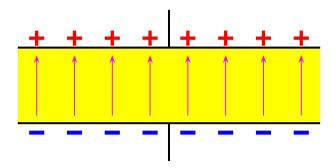
Let d be the distance between the plates and A the plates' area. Given the voltage V between the capacitor plates, the electric field inside the capacitor is approximately uniform
