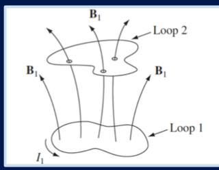
If the current in loop 1 changes, the flux through loop 2 will vary accordingly. The changing flux will induce an emf in loop 2
