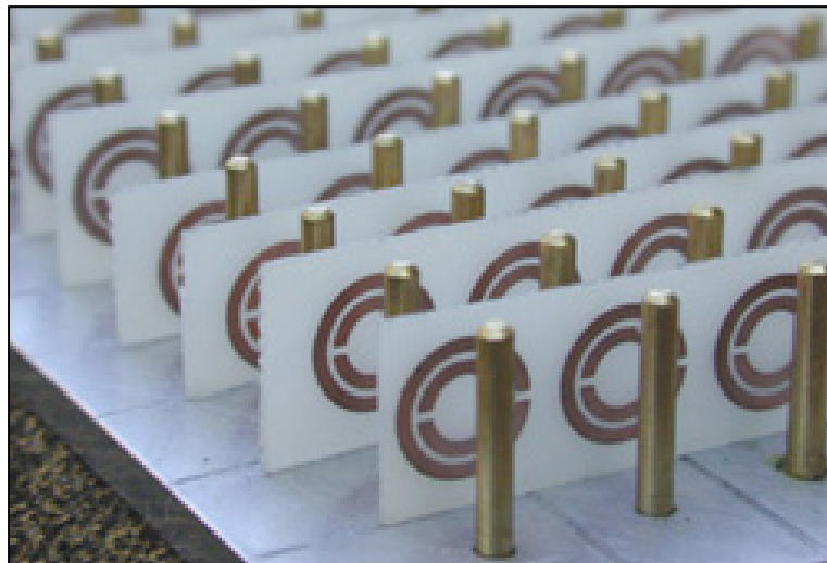
Figure 5-5. Wire and Split-Ring Structure Designed for the Megahertz Range
