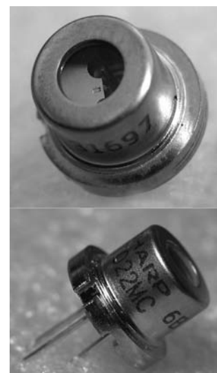
Figure 16 Two views of a packaged laser diode. The packaged diode is about 6 mm in diameter. The laser diode chip itself is located in the small rectangular depression visible in the mount shown in the top image. Courtesy of John Sohl. (Photo by Sheri Trbovich.)
