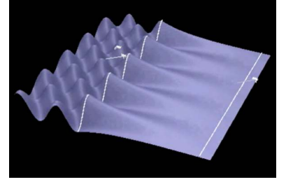
Figure 4.5 Animation showing frustrated total internal reflection.
