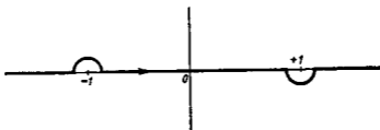
Fig. 11.5. The path of integration from -\infty to +\infty in the complex \mu plane.
