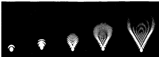
Fig. 9.8. Images in the Gaussian focal plane in the presence of coma \Phi = 0.3\lambda\rho^3 \cos \theta , \lambda\rho^3 \cos \theta , 2.4\lambda\rho^3 \cos \theta , 5\lambda\rho^3 \cos \theta , 10\lambda\rho^3 \cos \theta .
