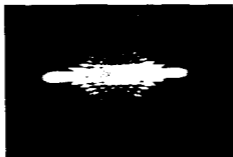
Fig. 9.11. Image in the plane containing a focal line, in the presence of primary astigmatism \Phi = 2.7\lambda\rho^2 \cos 2\theta .
