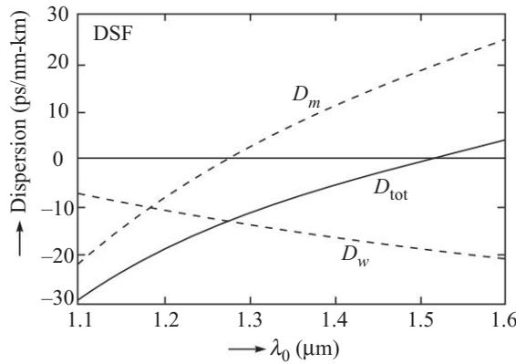
**Fig. 20.6** The wavelength dependence of  $D_m$ ,  $D_w$  and  $D_{tot}$  for a typical dispersion shifted fiber (DSF) with parameters as given in Problem 20.14. The zero dispersion wavelength is around 1550 nm.
