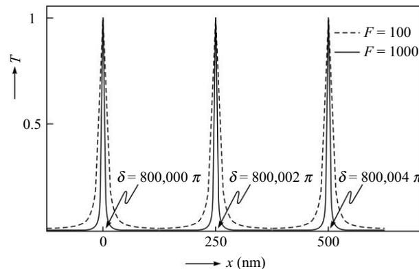
**Fig. 8.2** The variation of the transmission coefficient  $T$  with  $x$  for a monochromatic beam incident normally on a scanning Fabry-Perot interferometer; the solid curve corresponds to  $F = 1000$  and the dashed curve corresponds to  $F = 100$ .
