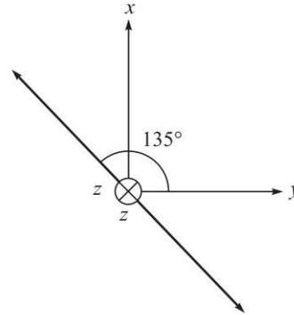
**Fig. 14.5** A linearly polarised wave making an angle of  $135^\circ$  with the  $y$ -axis; the propagation is in the  $+z$  direction.
