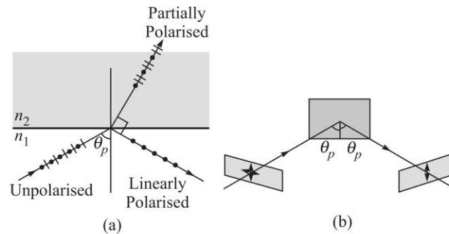
**Fig. 13.5** When an unpolarised beam of light is incident on a dielectric at the polarising angle [i.e., the angle of incidence is equal to  $\tan^{-1}(n_2/n_1)$ ] then the reflected beam is plane-polarised with its **E**-vector perpendicular to the plane of incidence. The transmitted beam is partially polarised. The dashed line in (b) is normal to the reflecting surface.
