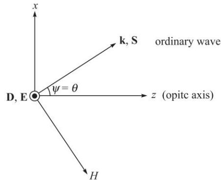
**Fig. 13.6** For the ordinary wave (in uniaxial crystals),  $\mathbf{D}$  and  $\mathbf{E}$  vectors are in the  $y$  direction;  $\mathbf{k}$  and  $\mathbf{S}$  are in the same direction in the  $x$ - $z$  plane and  $\mathbf{H}$  also lies in the  $x$ - $z$  plane.
