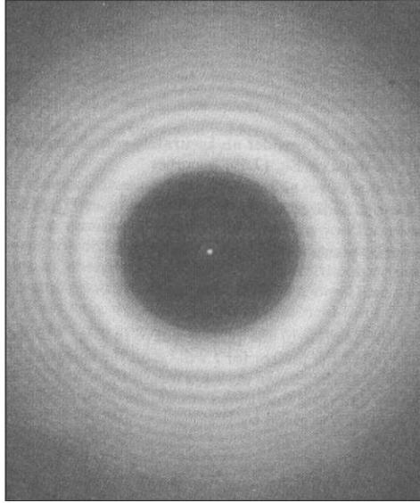
**Fig. 11.9** The Poisson spot at the center of the shadow of a one cent coin; the screen is 20 m from the coin and the source of light is also 20 m from the coin. Photograph from Ref. R: 1; used with permission from P. M. Rinard and American association of Physics Teachers.
