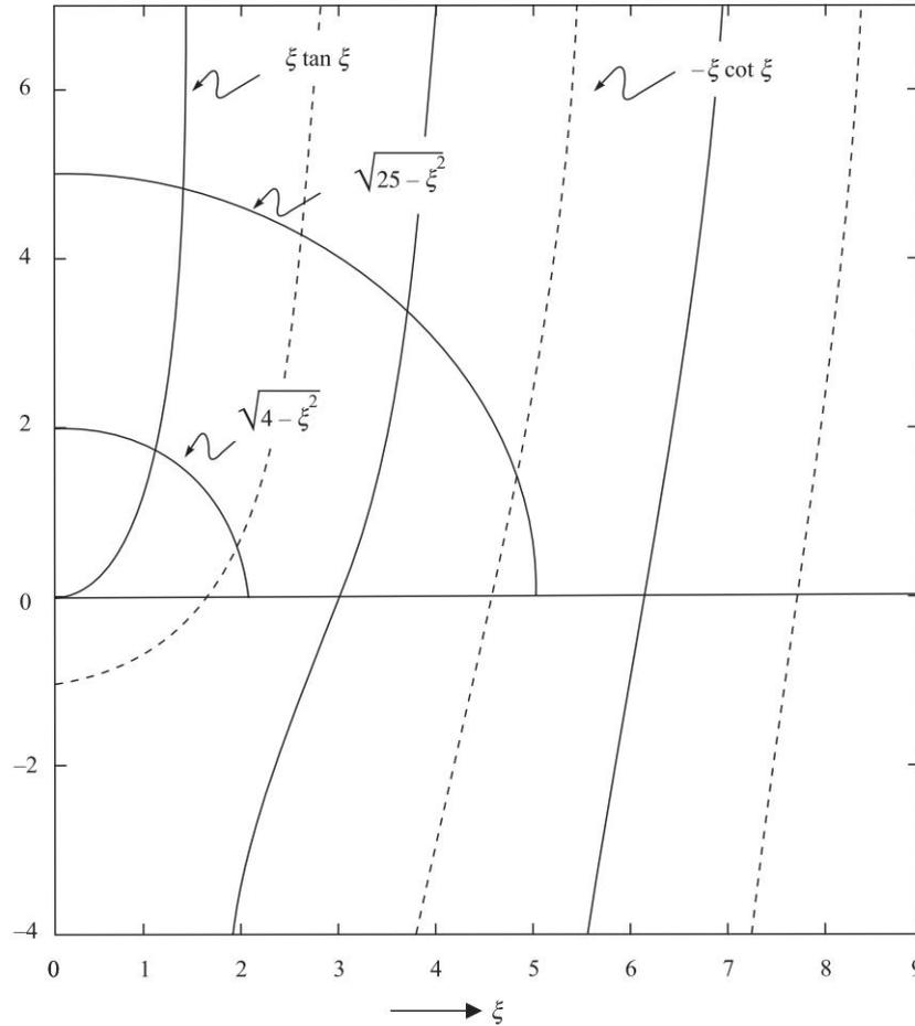
**Fig. 19.2** Variation of  $\xi \tan \xi$  (solid curve) and  $-\xi \cot \xi$  (dashed curve) as a function of  $\xi$ . The points of intersection of these curves with the quadrant of a circle of radius  $V/2$  determine the discrete propagation constants of the waveguide.
