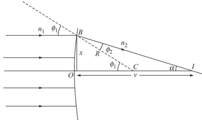
**Fig. 4.8** A parallel beam of light is incident on a spherical surface separating two media of refractive indices  $n_1$  and  $n_2$ . The point  $C$  represents the center of curvature of the refracting surface.
