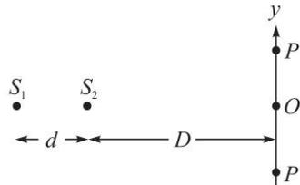
Fig. 6.6  $S_1$  and  $S_2$  represent two coherent sources.
