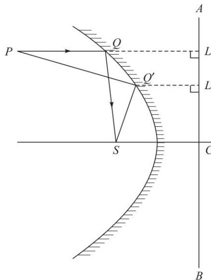
**Fig. 2.4** All rays parallel to the axis of a paraboloidal reflector pass through the focus after reflection (the line  $ACB$  is the directrix). It is for this reason that antennas (for collecting electromagnetic waves) or solar collectors are often paraboloidal in shape.
