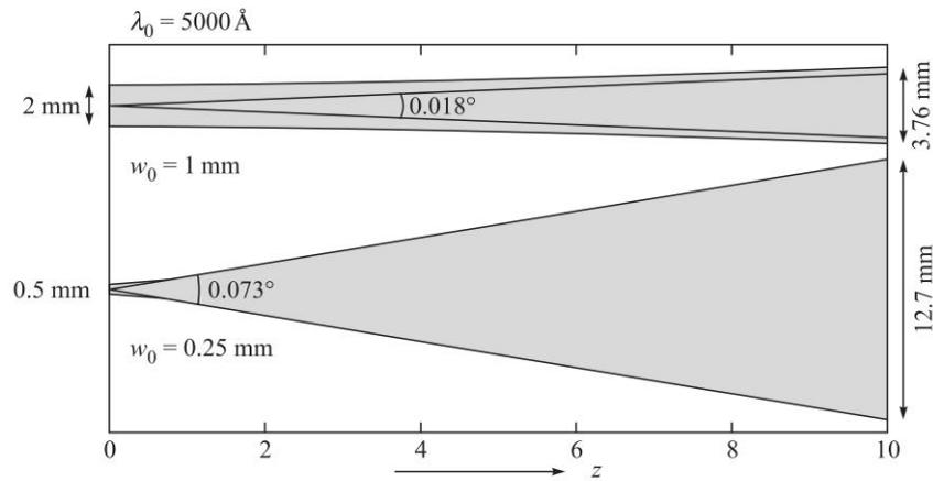
**Fig. 11.11** Diffraction divergence of a Gaussian beam whose phase front is plane at  $z = 0$ . The figure shows the increase in the diffraction divergence as the initial spot size is decreased from 1 mm to 0.25 mm; the wavelength is assumed to be 5000 Å.
