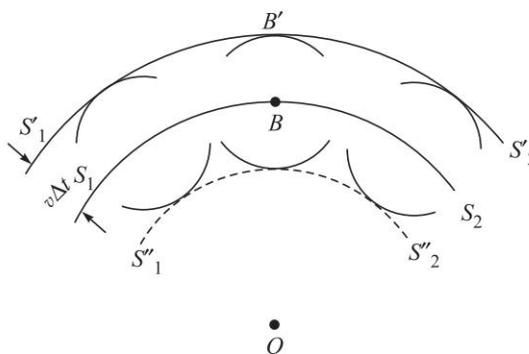
**Fig. 5.1** Huygens' construction for the determination of the shape of the wavefront, given the shape of the wavefront at an earlier time.  $S_1S_2$  is a spherical wavefront centered at  $O$  at a time, say  $t = 0$ .  $S'_1S'_2$  corresponds to the state of the wavefront at a time  $\Delta t$ , which is again spherical and centered at  $O$ . The dashed curve represents the backwave.
