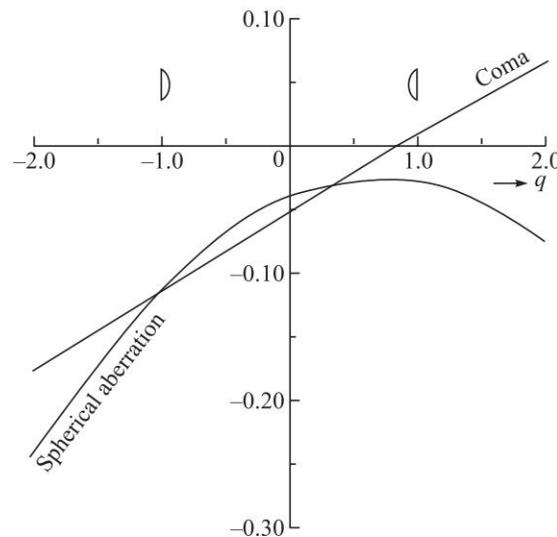
**Fig. 4.4** Variation of spherical aberration and coma with the shape factor of a thin lens with  $n = 1.5$ ,  $f = 40$  cm and  $h = 1$  cm. For calculating the coma we have assumed  $\tan \theta = 1$ , i.e., rays make an angle of  $45^\circ$  with the axis.
