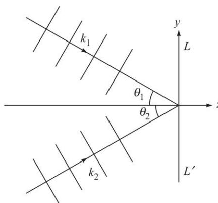
Fig. 6.7 Superposition of two plane waves on  $LL'$ .
