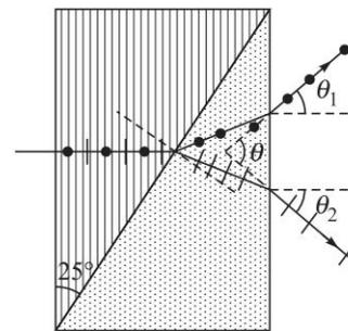
Fig. 13.15 A Wollaston prism. The lines and dots show the direction of the optic axis.
