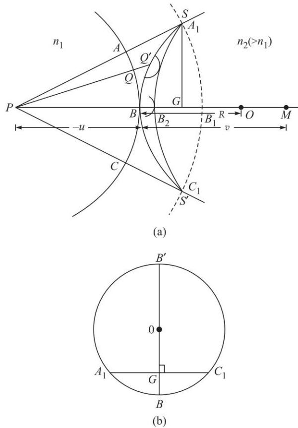
**Fig. 5.5** (a) Refraction of a spherical wave  $ABC$  (emanating from the point source  $P$ ) by a convex spherical surface  $SBS'$  separating media of refractive indices  $n_1$  and  $n_2 (> n_1)$ .  $A_1B_2C_1$  is the refracted wavefront, which is approximately spherical and whose center of curvature is at  $M$ . Thus  $M$  is the real image of  $P$ .  $O$  is the center of curvature of  $SS'$ . (b) The diameter  $B'OB$  intersects the chord  $A_1GC_1$  normally.
