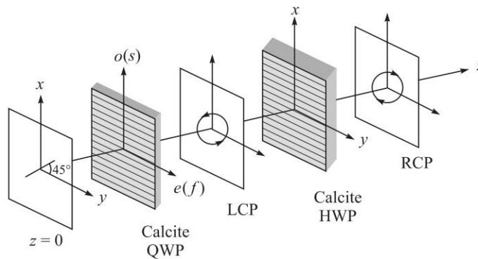
Fig. 14.3 A linearly polarised beam making an angle  $45^\circ$  with the  $y$ -axis gets converted to a LCP after propagating through a calcite QWP whose optic axis is along the  $y$ -axis as shown by lines parallel to the  $y$ -axis. Further, an LCP gets converted to a RCP after propagating through a calcite HWP; the optic axis of the HWP is also assumed to be along the  $y$ -direction.
