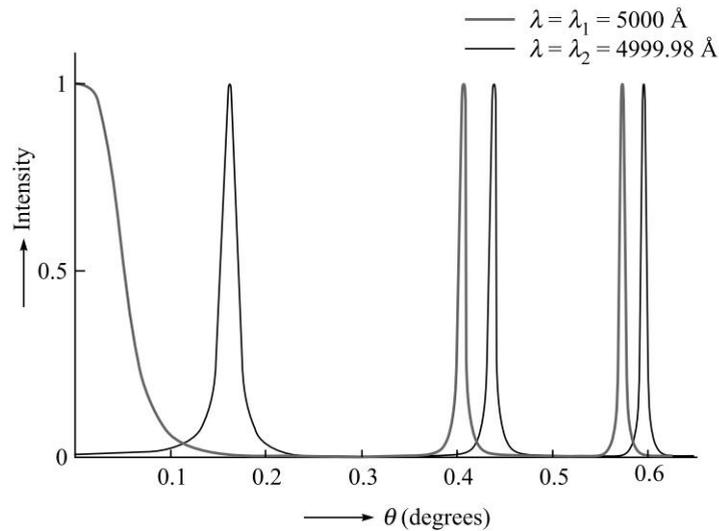
Fig. 8.6 The variation of intensity with  $\theta$  for a Fabry-Perot interferometer with  $n_f = 1$ ,  $h = 1.0 \text{ cm}$  and  $F = 400$ , corresponding to  $\lambda_0 = 5000 \text{ \AA}$  ( $= \lambda_1$ ) and  $\lambda_0 = 4999.98 \text{ \AA}$  ( $= \lambda_2$ ).
