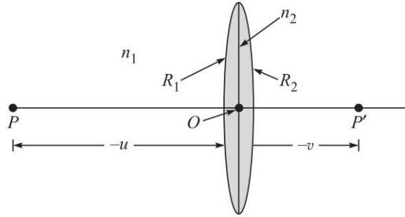
**Fig. 5.6** A thin lens made of a medium of refractive index  $n_2$  placed in a medium of refractive index  $n_1$ . The radii of curvatures of the two surfaces are  $R_1$  and  $R_2$ .  $P$  is the image (at a distance  $v$  from the point  $O$ ) of the point object  $P$  (at a distance  $-u$  from the point  $O$ ).
