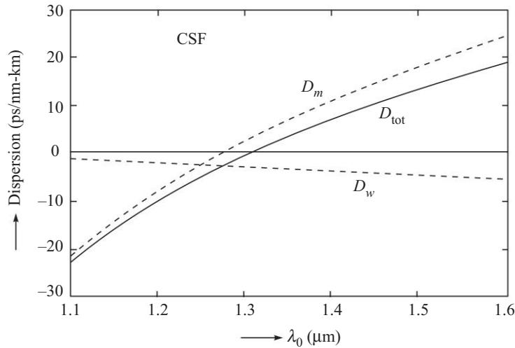
**Fig. 20.5** The wavelength dependence of  $D_m$ ,  $D_w$  and  $D_{\text{tot}}$  for a typical conventional single mode fiber (CSF) with parameters as given in Problem 20.13. The total dispersion passes through zero around  $\lambda_0 \approx 1300$  nm which is known as zero dispersion wavelength.
