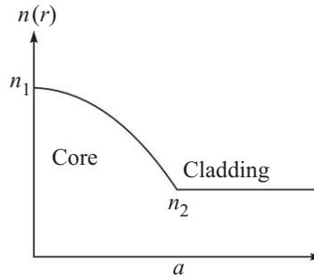
**Fig. 20.2** A cylindrically symmetric refractive index profile having a refractive index that decreases monotonically from a value  $n_1$  on the axis to a constant value  $n_2$  beyond the core-cladding interface  $r = a$ .
