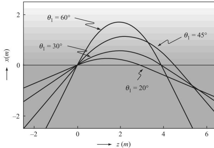
**Fig. 2.8** Parabolic ray paths (corresponding to  $\theta_1 = 20^\circ, 30^\circ, 45^\circ$  and  $60^\circ$ ) in a medium characterised by refractive index variation as given in Problem 2.9. The ray paths in the region  $x < 0$  are straight lines.
