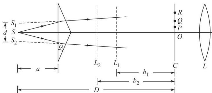
**Fig. 6.3** Fresnel's biprism arrangement.  $C$  and  $L$  represent the positions of the crosswires and the eyepiece respectively. In order to determine  $d$  one introduces a lens between the biprism and the crosswires;  $L_1$  and  $L_2$  represent the two positions of the lens where the slits are clearly seen.
