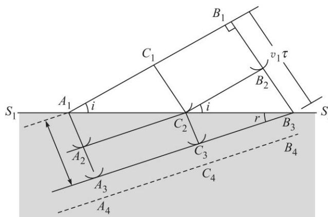
**Fig. 5.3** Refraction of a plane wavefront  $A_1B_1$  by a plane interface  $S_1S_2$  separating two media with different velocities of propagation of light  $v_1$  and  $v_2$  ( $<v_1$ );  $i$  and  $r$  are the angles of incidence and refraction respectively.  $A_2C_2B_2$  corresponds to the shape of the wavefront at an intermediate time  $\tau$ . Notice that  $r < i$ .
