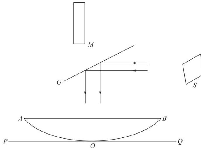
**Fig. 7.2** An arrangement for observing Newton's rings. Light from an extended source  $S$  is allowed to fall on a thin film formed between the plano-convex lens  $AOB$  and the plane glass plate  $POQ$ .  $M$  represents a traveling microscope.
