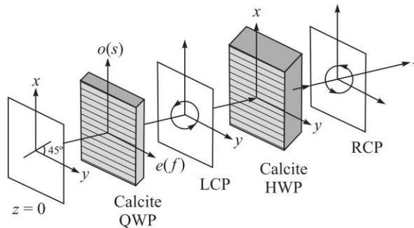
**Fig. 13.8** A linearly polarised beam making an angle  $45^\circ$  with the  $y$ -axis gets converted to a LCP after propagating through a calcite QWP whose optic axis is along the  $y$ -axis as shown by lines parallel to the  $y$ -axis. Further, an LCP gets converted to a RCP after propagating through a calcite HWP; the optic axis of the HWP is also assumed to be along the  $y$ -direction.
