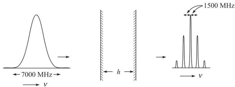
**Fig. 8.3** A beam having a spectral width of about 7000 MHz (around  $\nu_0 = 6 \times 10^{14}$  Hz) is incident normally on a Fabry-Perot etalon with  $h = 10$  cm and  $n_f = 1$ . The output has 5 narrow spectral lines.
