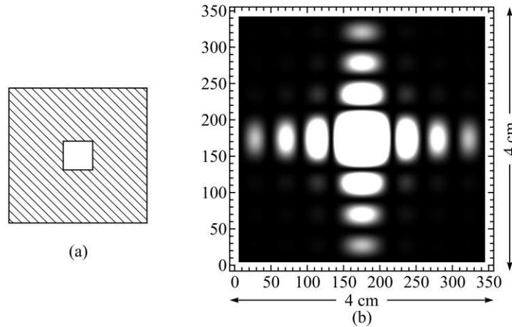
**Fig. 10.10** (a) A square aperture of side 0.01 cm. (b) The corresponding (computer generated) Fraunhofer diffraction pattern on a screen at a distance of 100 cm from the aperture;  $\lambda = 5 \times 10^{-5}$  cm.
