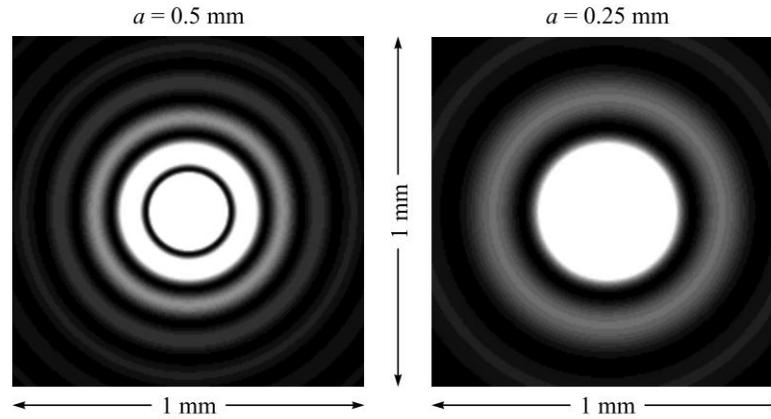
**Fig. 10.11** Computer generated Airy patterns; (a) and (b) correspond to  $a = 0.5$  mm and  $a = 0.25$  mm respectively at the focal plane of a lens of focal length 20 cm ( $\lambda = 0.5 \mu\text{m}$ ).
