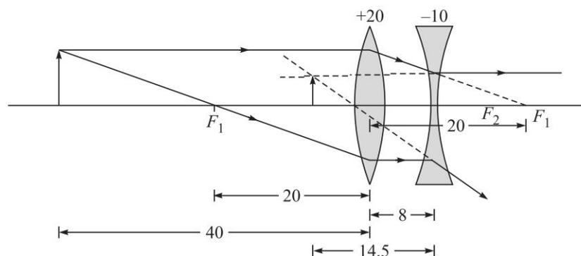
Fig. 1.9 A combination of two thin lenses.
