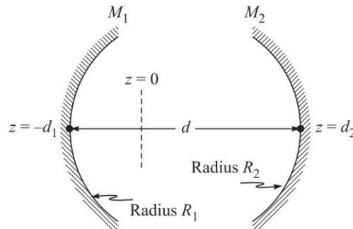
**Fig. 17.3** A resonator consisting of two spherical mirrors.
