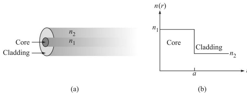
**Fig. 20.1** (a) A step index fiber is a cylindrical structure in which the refractive index is  $n_1$  for  $0 < r < a$  and  $n_2$  for  $r > a$  (b) The refractive index variation of a step index fiber.
