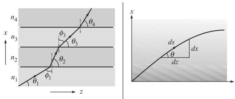
**Fig. 2.2** (a) In a layered structure, the ray bends in such a way that the product  $n_1 \sin \phi_1 = n_2 \sin \phi_2 = n_3 \sin \phi_3 = \dots$  remains constant. (b) For a medium with continuously varying refractive index, the ray path bends in such a way that the product  $n(x) \sin \phi(x) [= n(x) \cos \theta(x)]$  remains constant.
