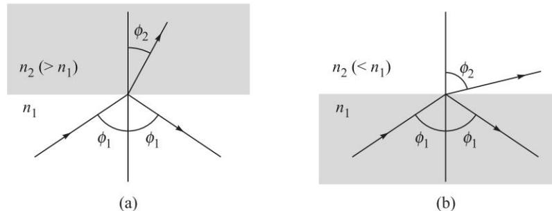
**Fig. 2.1** (a) For a ray incident on a denser medium, the ray bends towards the normal and the angle of refraction is less than the angle of incidence. (b) For a ray incident on a rarer medium, the ray bends away from the normal and the angle of refraction is greater than the angle of incidence. In each refraction, the Snell's law  $n_1 \sin \phi_1 = n_2 \sin \phi_2$  is obeyed.
