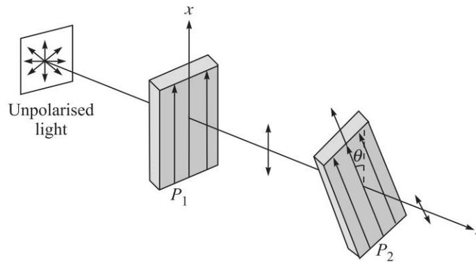
**Fig. 13.2** An unpolarised light beam gets  $x$ -polarised after passing through the polaroid  $P_1$ , the pass axis of the second polaroid  $P_2$  makes an angle  $\theta$  with the  $x$ -axis. The intensity of the emerging beam will vary as  $\cos^2 \theta$ .
