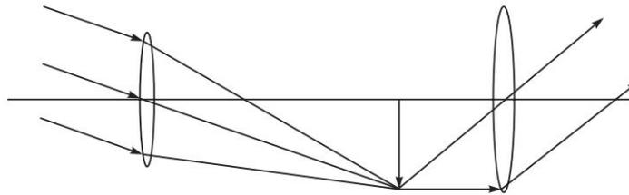
**Fig. 3.2** A telescope consisting of an objective lens and an eye piece. Parallel rays from a distant object get focused on the focal plane of the objective and the eye piece provides for magnification of the image.
