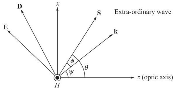
**Fig. 13.7** For the extraordinary wave (in uniaxial crystals),  $\mathbf{E}$ ,  $\mathbf{D}$ ,  $\mathbf{S}$  and  $\mathbf{k}$  vectors would lie in the  $x$ - $z$  plane and  $\mathbf{H}$  will be in the  $y$  direction.  $\mathbf{S}$  is at right angles to  $\mathbf{E}$  and  $\mathbf{H}$ ;  $\mathbf{D}$  is at right angles to  $\mathbf{k}$  and  $\mathbf{H}$ .
