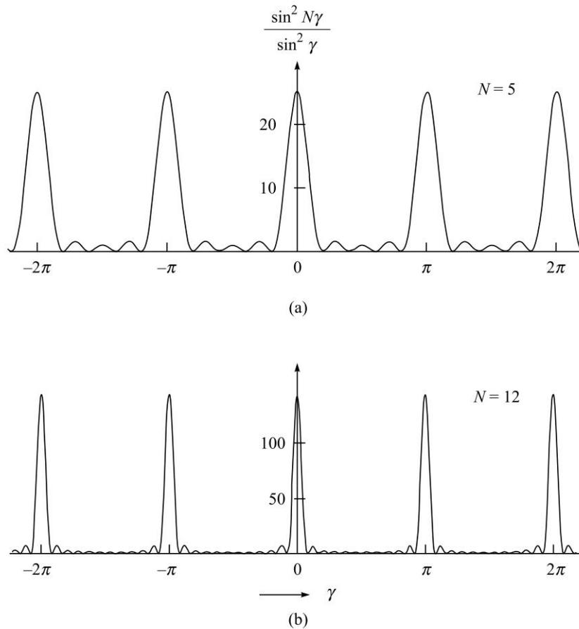
**Fig. 9.12** The variation of the function  $\sin^2(N\gamma)/\sin^2 \gamma$  with  $\gamma$  for  $N=5$  and  $12$ . As  $N$  becomes larger, the function would become more and more sharply peaked at  $\gamma = 0, \pm \pi, \pm 2\pi, \pm 3\pi, \dots$
