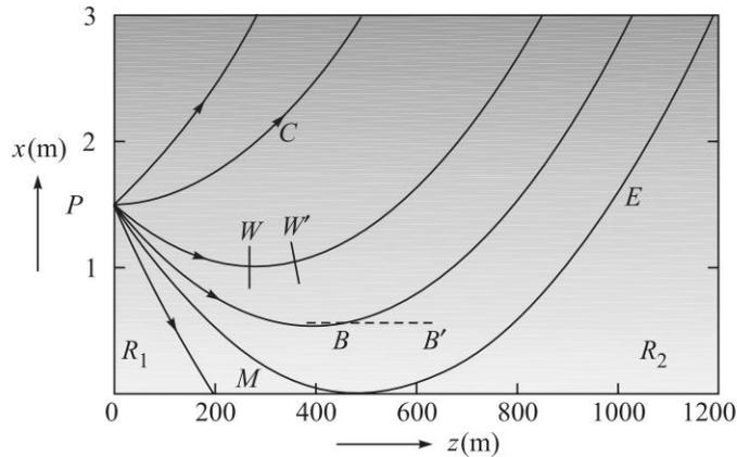
**Fig. 2.6** Ray paths in a medium characterised by a linear variation of refractive index [see Eq. (7)] with parameters as given in Problem 6(b). The object point is at a height of 1.5 m and the curves correspond to  $+0.2^\circ$ ,  $0^\circ$ ,  $-0.2^\circ$ ,  $-0.28^\circ$ ,  $-0.3486^\circ$  and  $-0.5^\circ$ . The shading shows that the refractive index increases with  $x$ .
