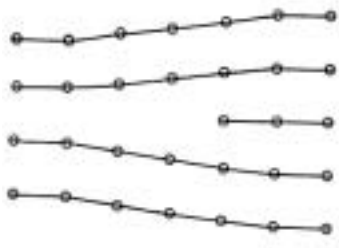
Fig. 9.12 Dislocation in a crystal. Here is a topological defect in a crystal. We can see that one of the rows of atoms on the right disappears halfway through our sample. The place where it disappears is a defect, because it doesn't locally look like a piece of the perfect crystal. It is a topological defect because it can't be fixed by any local rearrangement. No reshuffling of atoms in the middle of the sample can change the fact that five rows enter from the right, and only four leave from the left! The Burger's vector of a dislocation is the net number of extra rows and columns, combined into a vector (columns, rows).
