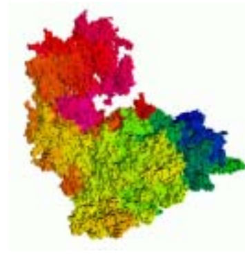
Fig. 12.2 A medium-sized avalanche (flipping 282,785 domains) in a model of avalanches and hysteresis in magnets (see exercises 8.12, 12.10 and figure 12.14). The shading depicts the time evolution: the avalanche started in the dark region in the back, and the last spins to flip are in the upper, front region. The sharp changes in shading are real, and represent sub-avalanches separated by times where the avalanche almost stops (see figure 8.24).
