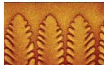
Fig. 11.16 Dendrites. Crystals growing into a melt will typically not grow compactly: the tips grow faster than the grooves. Here is shown some crystals growing into a melt in a thin film being pulled through a temperature gradient [12].
