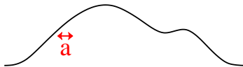
Fig. 2.4 We suppose the step sizes \ell are small compared to the broad ranges on which \rho(x) varies, so we may do a Taylor expansion in gradients of \rho .
