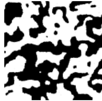
Fig. 10.1 The 2-D square-lattice Ising model, quenched (abruptly cooled) from high temperatures to zero temperature [103]. The model quickly separates into local blobs of up and down spins, which grow and merge, coarsening to larger blob sizes (section 11.3.1).
