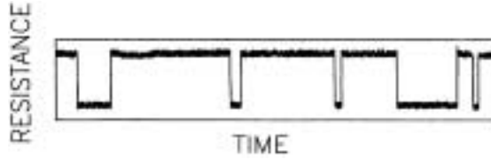
Fig. 10.15 Telegraph Noise in a metallic nanobridge. Resistance versus time R(t) for a copper constriction, from reference [87]. We label \alpha the state with low resistance R_\alpha , and \beta the state with high resistance R_\beta . The two states probably represent a local shift of an atom or a small group of atoms in the constriction from one metastable state to another.
