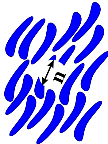
Fig. 9.5 Nematic liquid crystals are made up of long, thin molecules that prefer to align with one another. (Liquid crystal watches are made of nematics.) Since they don't care much which end is up, their order parameter is not a vector \hat{n} along the axis of the molecules, but is instead a unit vector up to the equivalence \hat{n} \equiv -\hat{n} .
