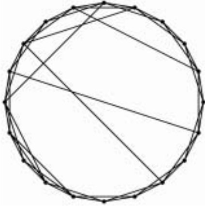
Fig. 8.16 Small world network, with L = 20 , Z = 4 , and p = 0.2 . 55
