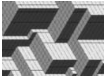
Fig. 11.14 Logarithmic Growth of an Interface. A simplified model of an interface perpendicular to a body diagonal in the Ising model of figure 11.13, [113]. Notice that the interface is lowering its energy by poking out into facets along the cubic directions (a kind of facet coarsening). This process gets much slower as the faces get longer, because the energy barrier needed to flip a face grows linearly with its length.
