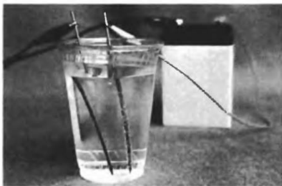
Figure 5.3. To separate water into hydrogen and oxygen, just run an electric current through it. In this home experiment the electrodes are mechanical pencil leads (graphite). Bubbles of hydrogen (too small to see) form at the negative electrode (left) while bubbles of oxygen form at the positive electrode (right).
