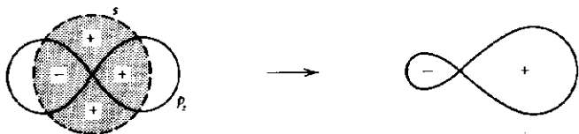
Fig. 21-5. Combination of s and p_z orbitals leading to unsymmetric wave function.
