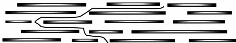
Fig. 12.20. The presence of nanoparticles in the polymer matrix imposes a tortuous path on the diffusing species.
