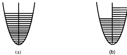
Fig. 3.6. (a) The closely spaced (“quasicontinuous”) energy levels according to the free electron theory; the energy levels up to the Fermi energy are occupied in the absence of the electric field (b) when an electric field is applied, some electrons acquire higher velocity and move to higher energy levels while the others lose speed giving a redistribution of the occupied states as shown.
