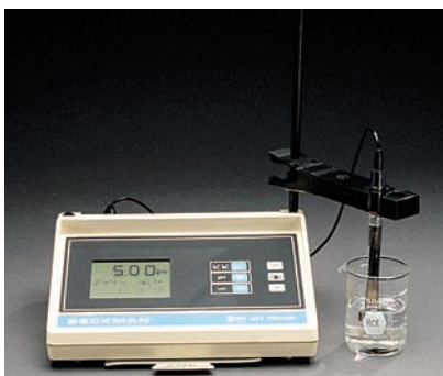
FIGURE 18.7 Methods for measuring the pH of an aqueous solution. A , A few drops of the solution are placed on a strip of pH paper, and the color is compared with the color chart. B , The electrodes of a pH meter immersed in the test solution measure [\text{H}_3\text{O}^+] . (In this instrument, the two electrodes are housed in one probe.)
