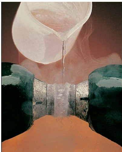
FIGURE 11.21 The paramagnetic properties of O_2 . Liquid O_2 is attracted to the poles of a magnet because it is paramagnetic, as MO theory predicts. A diamagnetic substance would fall between the poles.
