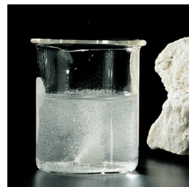
FIGURE 19.11 Test for the presence of a carbonate. When a mineral that contains carbonate ion is treated with strong acid, the added \text{H}_3\text{O}^+ shifts the equilibrium position of the carbonate solubility. More carbonate dissolves, and the carbonic acid that is formed breaks down to water and gaseous \text{CO}_2 .
