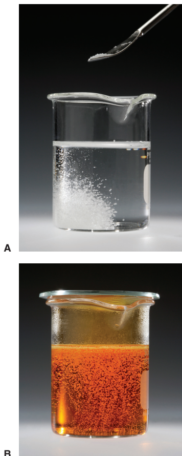
Figure 16.20 The catalyzed decomposition of \text{H}_2\text{O}_2 . A , A small amount of \text{NaBr} is added to a solution of \text{H}_2\text{O}_2 . B , Oxygen gas forms quickly as \text{Br}^-(aq) catalyzes the \text{H}_2\text{O}_2 decomposition; the reaction intermediate, \text{Br}_2 , turns the solution orange.
