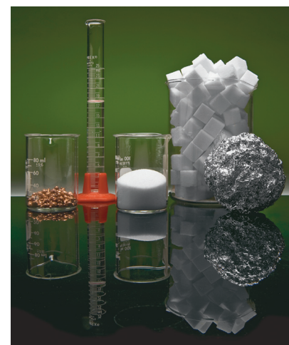
Figure 3.1 One mole ( 6.022 \times 10^{23} entities) of some familiar substances. From left to right: 1 mol of copper (63.55 g), of liquid H 2 O (18.02 g), of sodium chloride (table salt, 58.44 g), of sucrose (table sugar, 342.3 g), and of aluminum (26.98 g).
