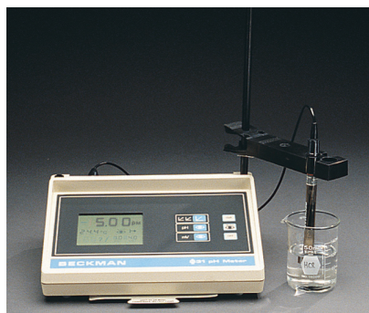
Figure 18.6 Methods for measuring the pH of an aqueous solution. A , pH paper. B , pH meter.
