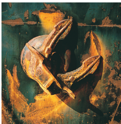
Figure 21.21 Enhanced corrosion at sea. The high ion concentration of seawater enhances the corrosion of iron in hulls and anchors.
