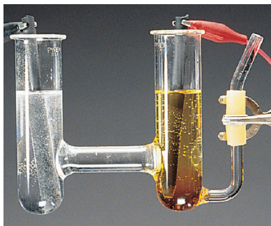
Electrolysis of aqueous KBr.
