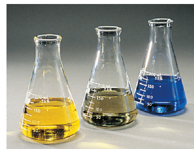
Figure 19.6 The color change of the indicator bromthymol blue.
