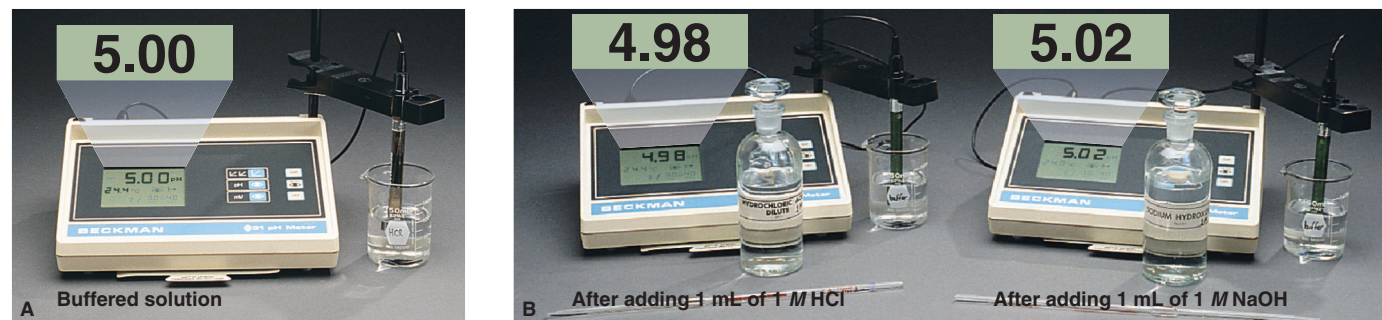
Figure 19.2 The effect of adding acid or base to a buffered solution. A , A 100-mL sample of an acetate buffer (1 M \text{CH}_3\text{COOH} mixed with
