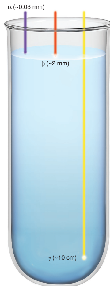
Figure 23.7 Penetrating power of radioactive emissions.
