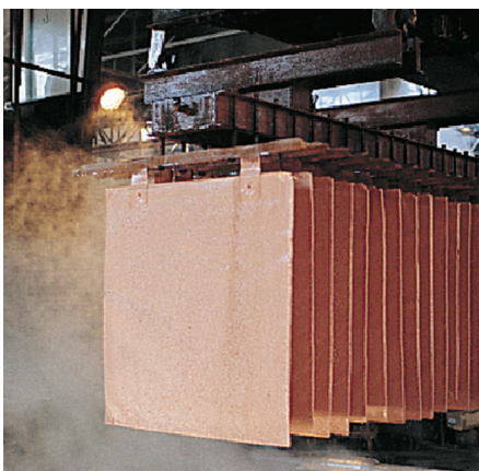
Figure 21.28 The electrorefining of copper.
