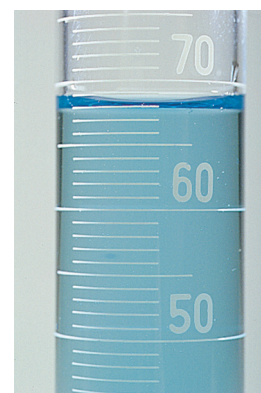
Figure 1.8 Significant figures and measuring devices. The mass measurement (6.8605 g) has more significant figures than the volume measurement (68.2 mL).
