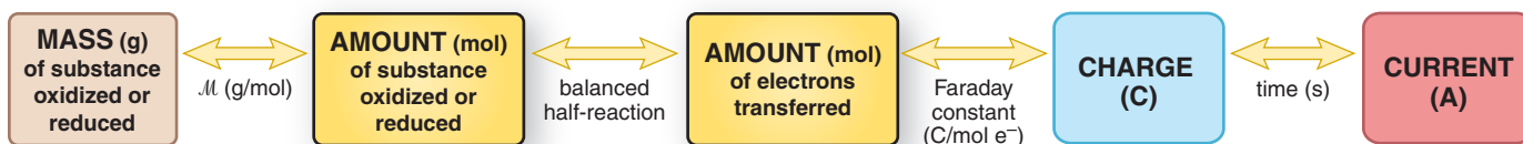
Figure 21.30 A summary diagram for the stoichiometry of electrolysis.
