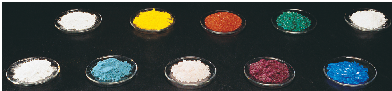
Figure 22.6 Colors of representative compounds of the Period 4 transition metals. Staggered from left to right, the compounds are scandium oxide ( white ), titanium(IV) oxide ( white ), vanadyl sulfate dihydrate ( light blue ), sodium chromate ( yellow ), manganese(II) chloride tetrahy-
