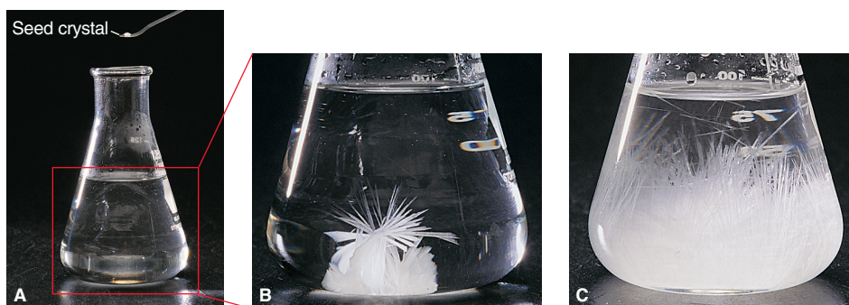
Figure 13.8 Sodium acetate crystallizing from a supersaturated solution. When a seed crystal of sodium acetate is added to a supersaturated solution of it ( A ), solute begins to crystallize ( B ) and continues until the remaining solution is saturated ( C ).
