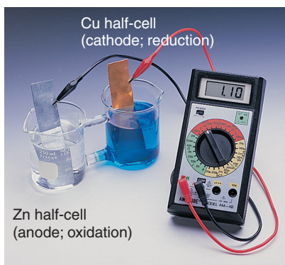
Figure 21.6 Measuring the standard cell potential of a zinc-copper cell.
