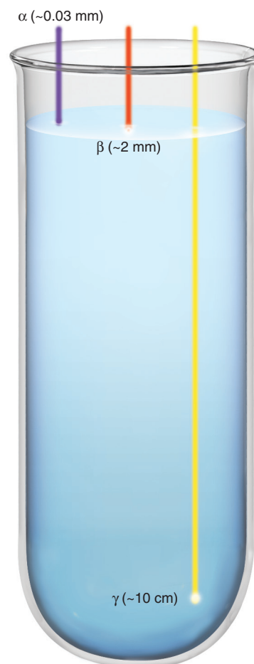
Figure 23.7 Penetrating power of radioactive emissions.
