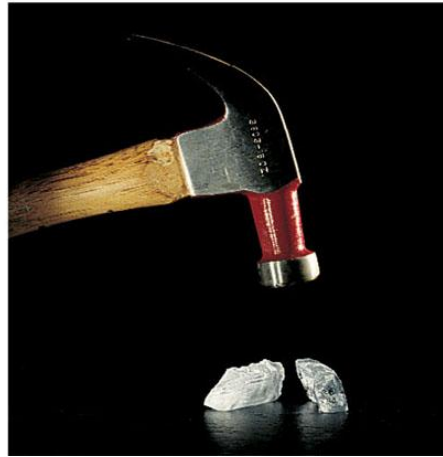
Figure 9.8 Why ionic compounds crack.
