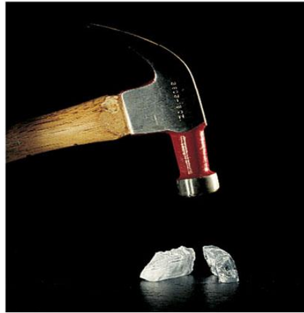
Figure 9.8 Why ionic compounds crack.
