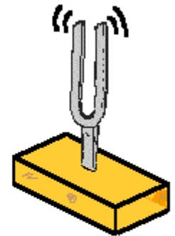
The tines of a tuning fork vibrate; its base is fixed. This is another example of an inverted pendulum.
