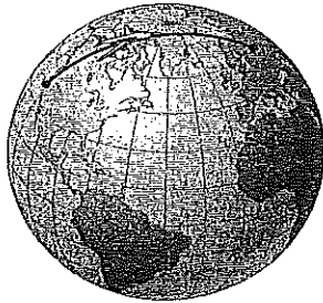
Figure 2.1 The shortest path between two points on a sphere is an arc of a great circle (a circle whose center is the center of the sphere and whose radius is the radius of the sphere, e.g., the equator).
