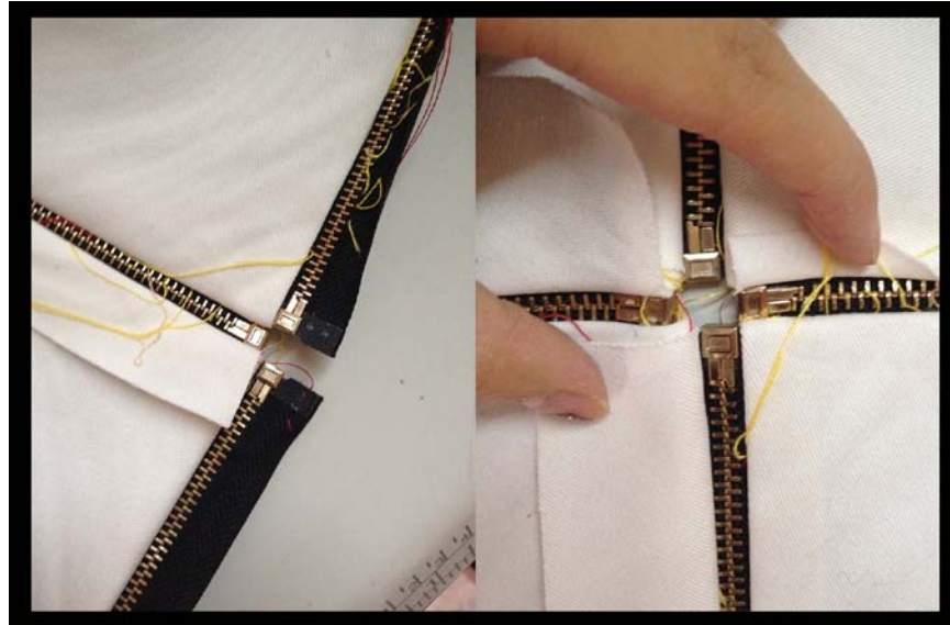
Figure 7.1. Sample making for zipper cross-connection technique
