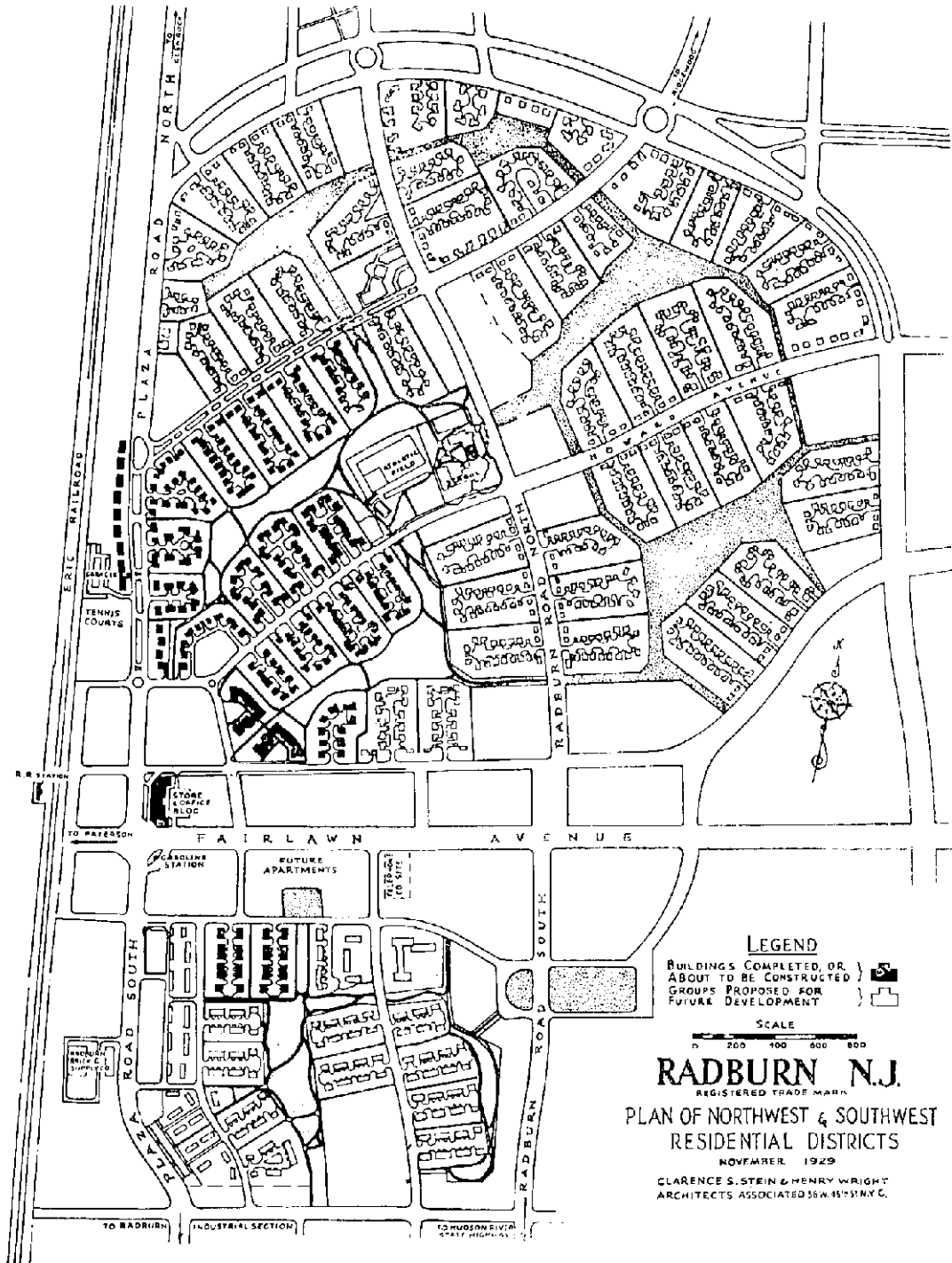
Plate 38 Plan for Radburn, New Jersey, 1929. Architects Clarence Stein and Henry Wright responded to the automobile by designing cities with a separation between pedestrian and traffic arteries, superblocs, and separate city areas with strong neighborhood identity. Their plan for Radburn, New Jersey, has inspired generations of planners.
