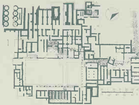
81 Mallia. Plan of the palace Middle of second millennium B.C. The palaces at Mallia, Hagia Triada and Phaestos were complexes of rooms arranged round a series of inner courtyards, a form already familiar elsewhere in the Near East.
