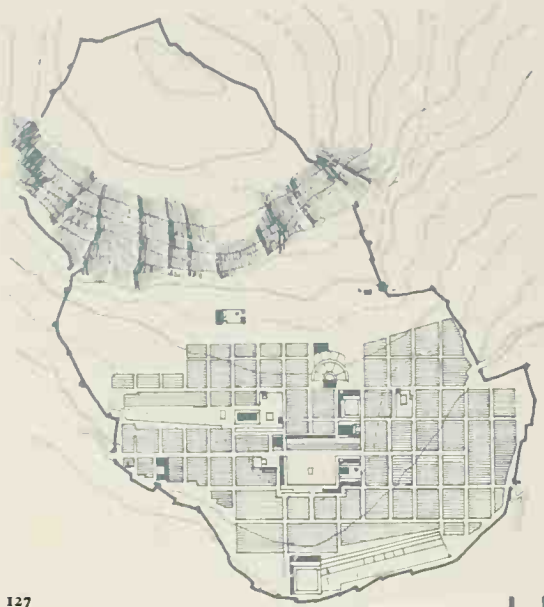
127 Plan of Priene Third century B.C. The town wall follows the natural contour of a rocky outcrop. The streets are laid out on a rectangular grid.
