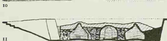
11 Section through a tomb at Ur End of third millennium B.C. An early and skilful use of untrimmed stone blocks for the construction of corbelled vaults.
