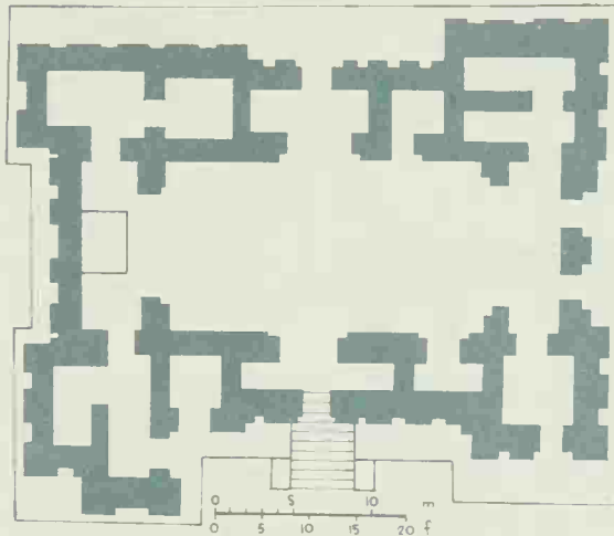
9 Plan of temple VII at Eridu. c. 3000 B.C. A late building in the Al'Ubaid series at Eridu. Already standing on its own platform, the central shrine or cella is now flanked by subsidiary chambers and the façade ornamented with buttresses.
