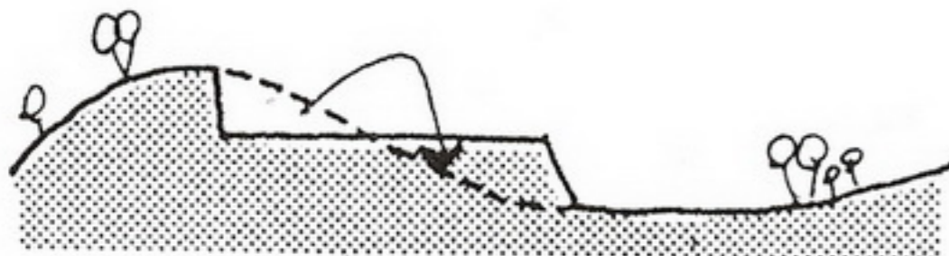
CUT = FILL FOR BUILDING PLATFORM
