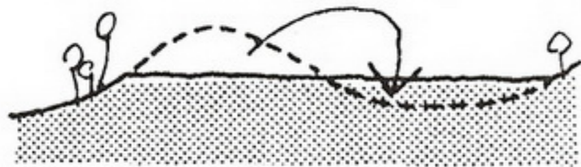
LEVEL SITE WITH CUT AND FILL
