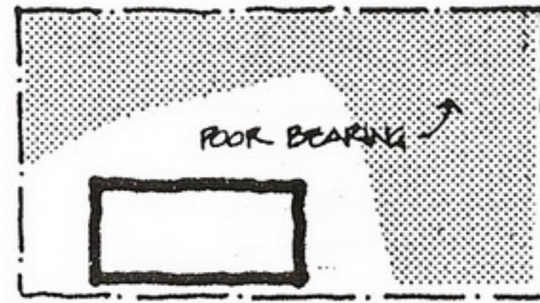
AVOID POOR SOIL BEARING
