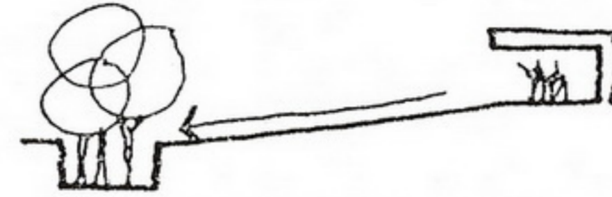
SLOPE EXTERIOR USE AREAS FOR POSITIVE DRAINAGE
