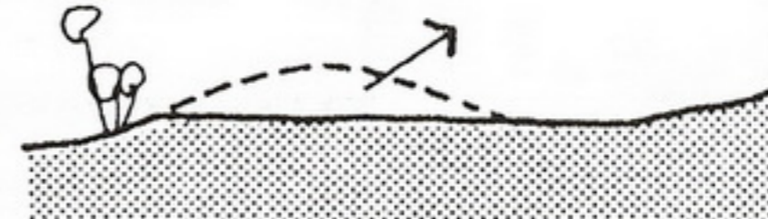
LEVEL WITH CUT AND REMOVE
