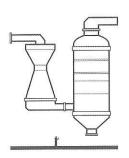
Scrubbers are filters that reduce the acidic components of the flue gas. They are towers where water is sprayed down into the upward-traveling flue gases. In the typical configuration, there is an acidic scrubber to remove HCI & HF and a neutral one for the removal of SO<sub>2</sub>.
